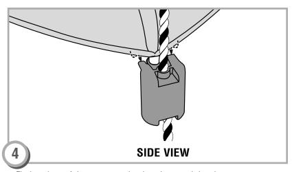
· Fit the edges of the canopy under the tab on each bracket.
